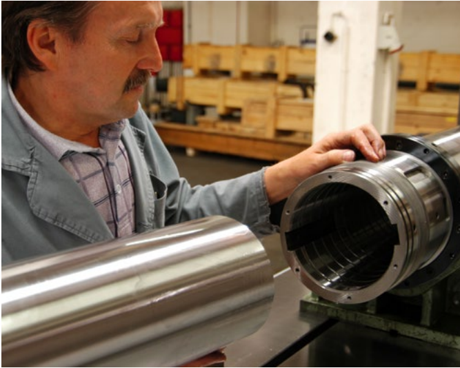
Boring spindle assembly with hollow spindle ground across the entire interior length and boring spindle paired to lubricant film thickness
