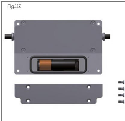
1. Unscrew the battery compartment at the rear of the electronics housing.
